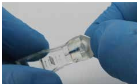
The silicon cap is removed to take the cover screw from the box.
